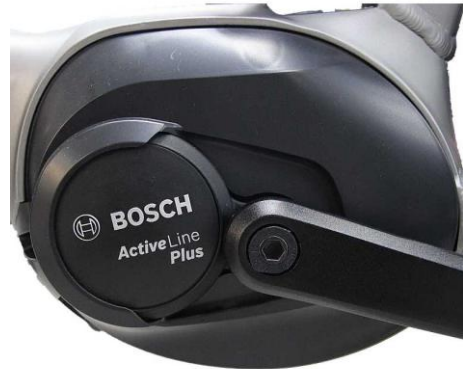
Bosch Active Plus max. 50 Nm
